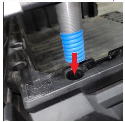
5. Route the wire from the topper down through the rectangular hole near the left rear of the cargo box, making sure the wire lays in the cutout to avoid pinching the wiring.
