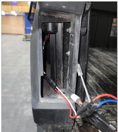
8. Once the topper is resting on the box, tighten the four anchors by hand (by turning the round eyelet clockwise) until they are snug.
