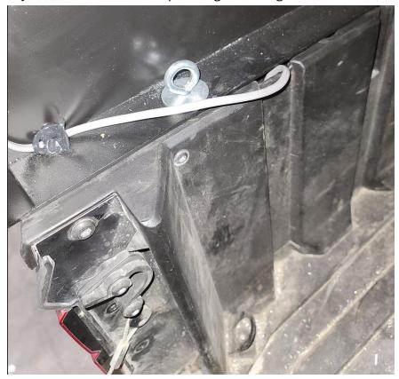
6. Accessing the topper connector from the rear (via the taillight opening), connect the rubber 2 wire connectors between the topper and the recently installed jumper harness. Before further assembly, test the wiring by turning the key to accessory (taillights should turn on) and turning on the interior light via the switch on the bottom of the light. After testing the light, turn the key off and proceed to the next step.
